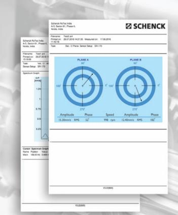
Measurement of overalls and frequency analysis
